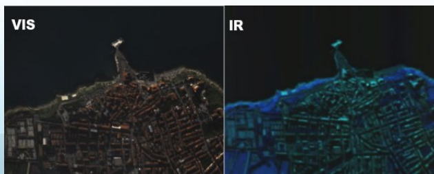
Coastline acquisitions using imaging spectrographs at 400-1000nm and 1000-2500nm
