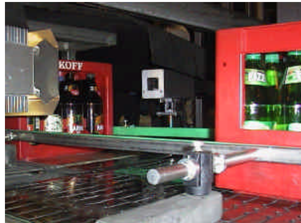
Figure 6. On-line crate sorting. Halogen light source on the left upper corner, ImSpector V7 and CCD camera looking from the square window on the center.
