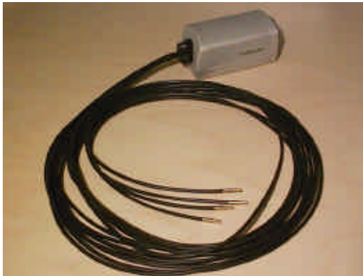
Figure 9. Standard PGP imaging spectrograph equipped with 4-legged fiberoptics, and schematic of a multitrack spectrometer.
