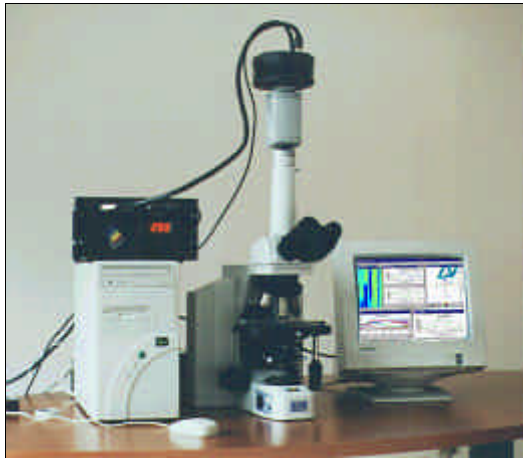
Figure 8. The direct sight spectrograph coupled to a standard microscope, and an example of ink recognition by spectral microscopy.
