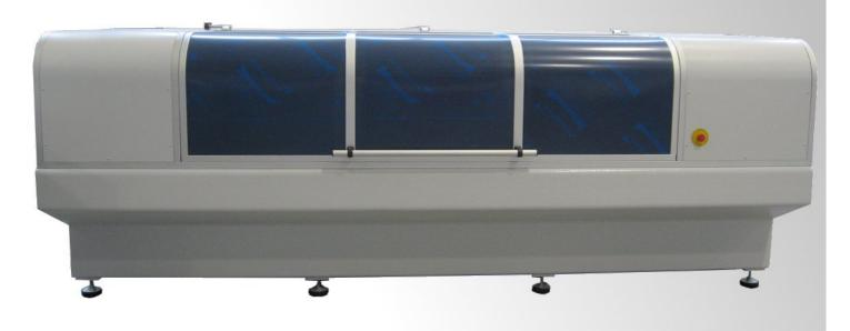
LLE allows to engrave a rotary trextile nickel screen through laser polymerization of a photosensitive emulsion totally chrome free.
