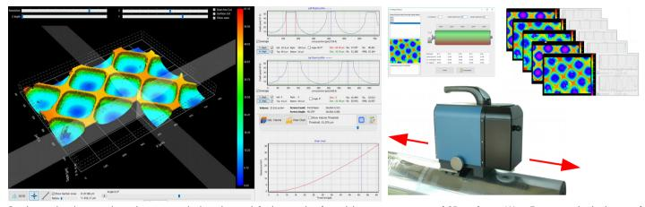
Our latest development is an instrument designed to satisfy the needs of precision measuremeant of 3D surfaces. WaveRunner embeds the art of high quality microscopy and interferometry since it can be used simultaneosly as a microscope or an interferometer. WaveRunner and the software InterferoLAB® can perform the following functions:
